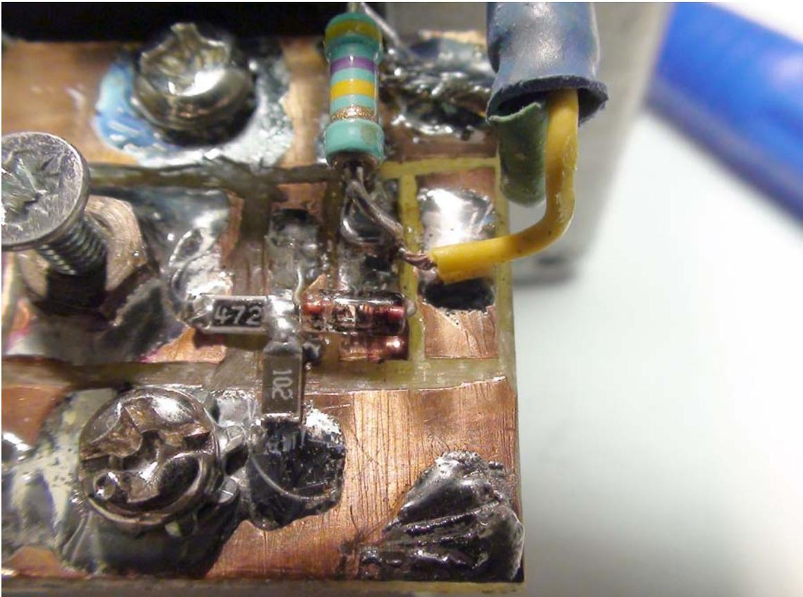
**Photo 3: Sampling PCB showing the smd resistors and diode. Tracks were cut with a Dremel disc.**
