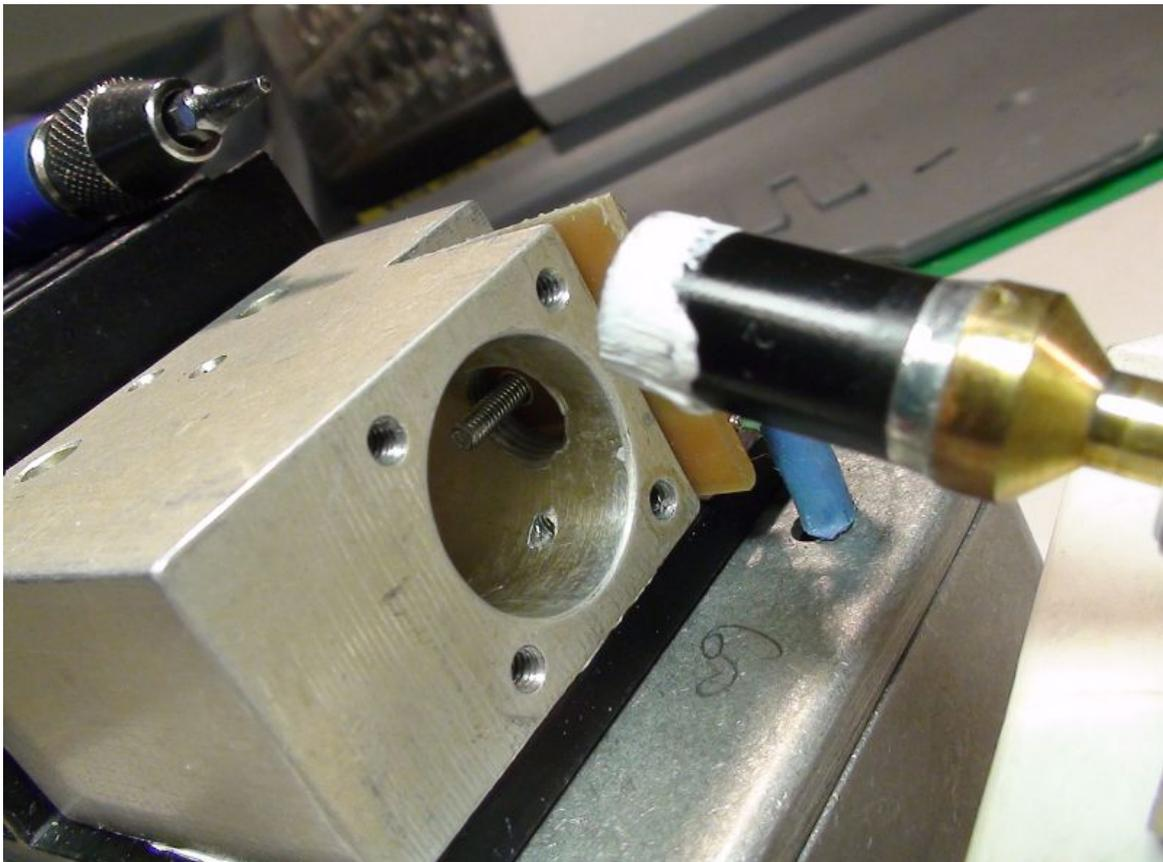
**Photo 4: Load resistor. Note the sampling screw visible through the side hole. This could have been placed more centrally.**
