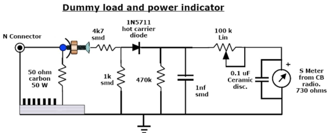
**Fig. 1 Circuit diagram of dummy load and power indicator.**
