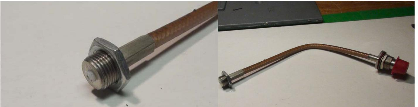
**Photo 6 & 7:** Here you see the original sampling cable that came with the load. The end of the centre conductor is trimmed and the coupling is adjusted by the screw and locking nut. This was removed and replaced with my sampling PCB.
