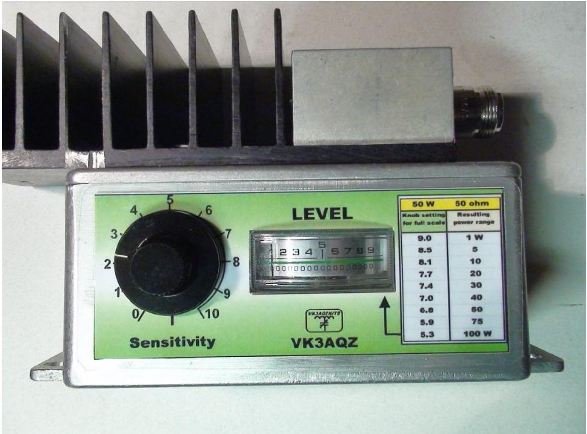
Photo 1: Front of unit showing the CB S meter, sensitivity pot and power chart.
