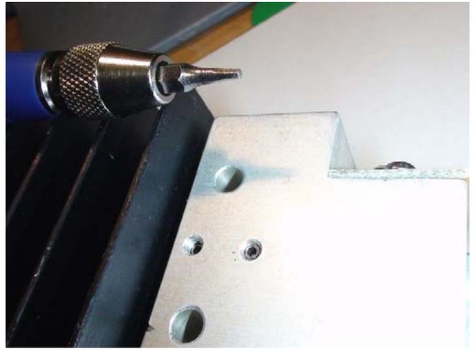
**Photo 4 & 5:** The earth end of the load resistor is held in place by a small grub screw (1.3mm hex key). A second grub screw holds a small bullet which is inserted up against the load resistor end. The white grease is heat conducting compound.
