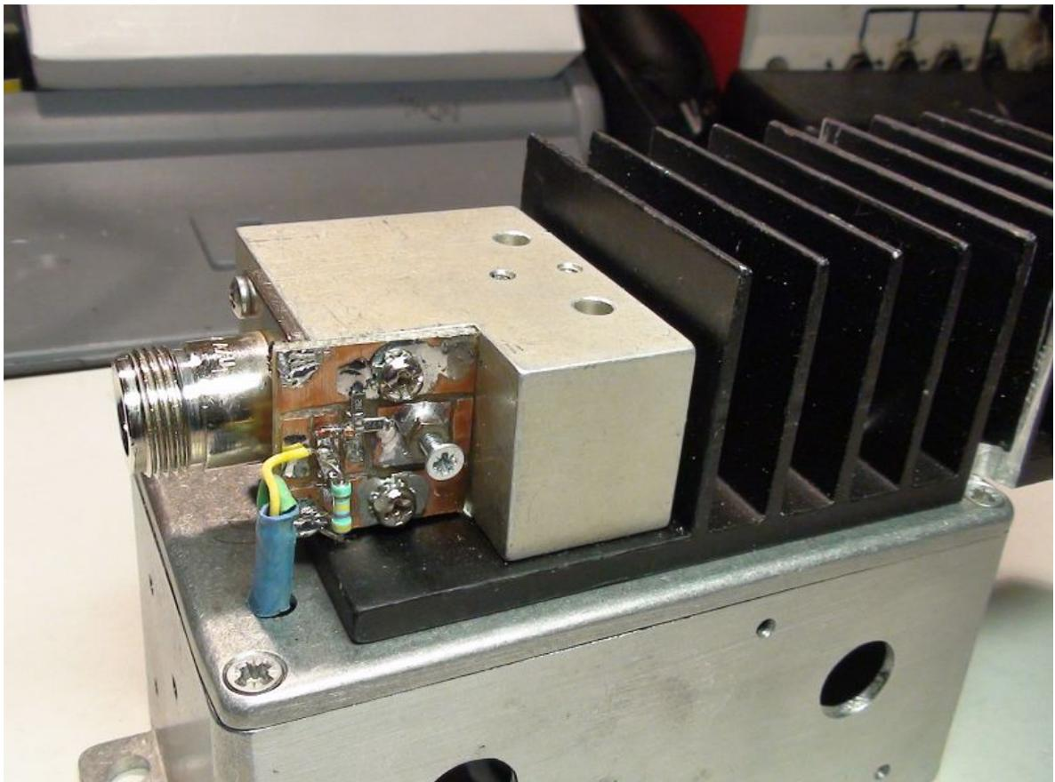
Photo 2: Sampling PCB attached to the load resistor mounting block.
