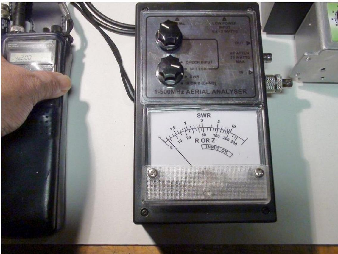
Photo 8 & 9: The VK5JST analyzer used to check the load at 432MHz with the sampling screw in contact with the load resistor (SWR 1.5:1), and then not in contact with the load resistor (SWR around 1.2:1).
